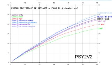
Figure 8: All test currents conducted with PSY2V2 are meanly better than the existing 100 m current: 6 % of improvement for the under-Ekman current over 100 m Current
