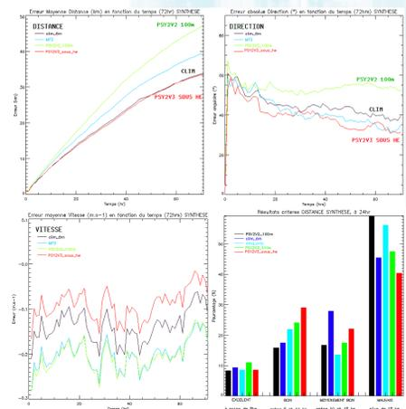
Figure 9: Summary of the mean results obtained in terms of distance, velocity and direction errors, between the replacement system PSY2V3 under Ekman current, the previous system PSY2V2 100m current, MFS system and the climatologic forcing.
