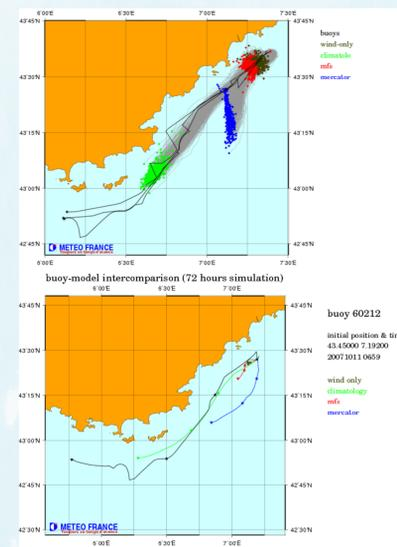
Figure 5: Example of a 72hr simulation, drifter n° 60212, different oceanic forcings evaluation.
