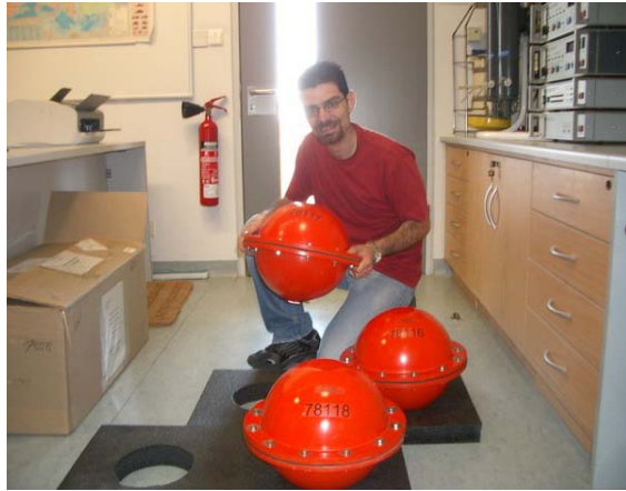
Argosphere oil-emulating surface drifters used in the E. Med experiment
